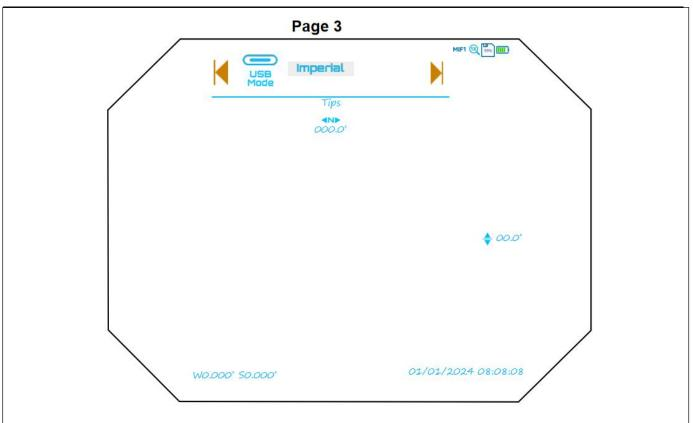
C) In page 3 the status bar is located in the upper portion of the screen, displays information about the actual operation state of the sight, from left to right in turn as follows:
